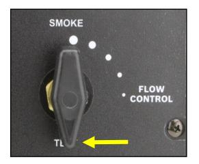
**TEST**: Delivers non-smoke air and a very accurate flow meter reading. This setting is for determining if a leak exists and how large it is.
