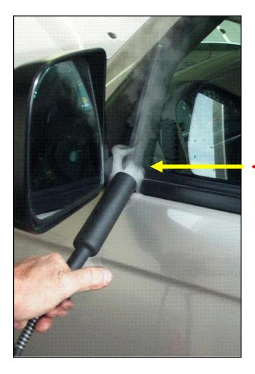
Smoke distrubance pinpoints the leak
